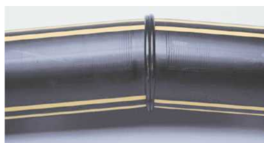
Unacceptable connection of pipes
